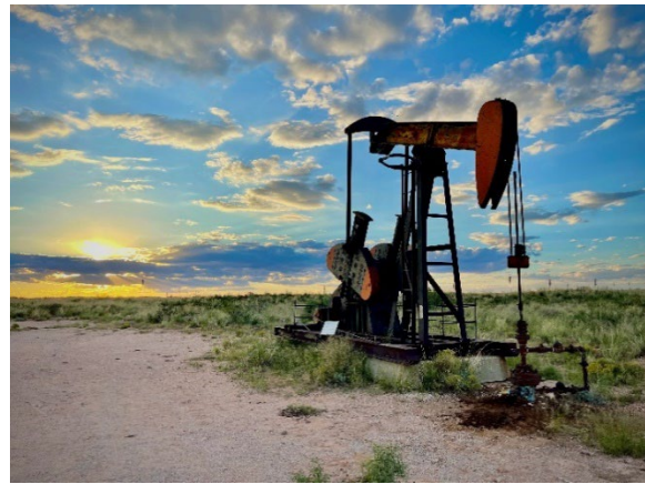
Orphan well prior to plugging.
