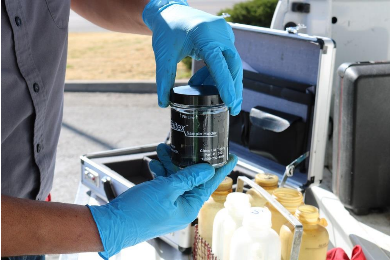
Cutline: The New Mexico Department of Agriculture Standards and Consumer Services Division performs regulatory activities under the authority of the Petroleum Products Standards Act. As part of these activities, petroleum inspectors test and screen fuel to ensure the octane and ethanol content is correct. (Photo courtesy New Mexico Department of Agriculture)
