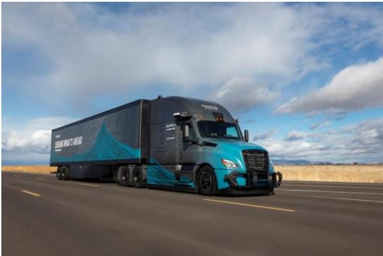
*Torc Robotics and Daimler Trucks are testing self-driving trucks near Albuquerque*
